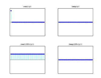
Figure 8.5. FFT of the first unit vector is constant
