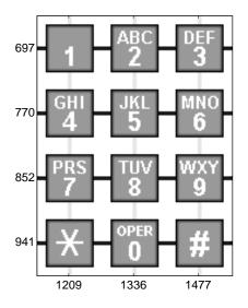
The tone generated by the button in position (k, j) is obtained by superimposing the two fundamental tones with frequencies fr(k) and fc(j).
