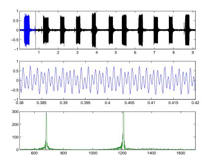
Figure 8.4. The first segment and its FFT
