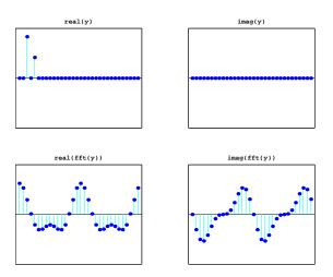
Figure 8.7. FFT is the sum of two sinusoids
